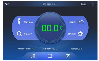
In the home page, it can display the real-time internal temperature, ambient temperature, set point, input voltage, backup system state (optional), network state, electromagnetic lock state (optional), user login status, freezer health status, temperature graph, and message/ note book, etc.. •Icon of real-time internal temperature:
