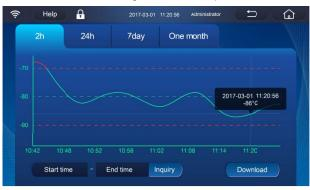
[2h] It can be used to quickly view the temperature graph of the last 2 hours, with the default value of 2 h(the default display range of graph can be set in the operation settings);
